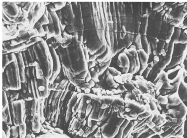
Figure 10 Scanning electron microscopy of the YSZ deposit plasma sprayed with the 30-particle-size-range powder.
